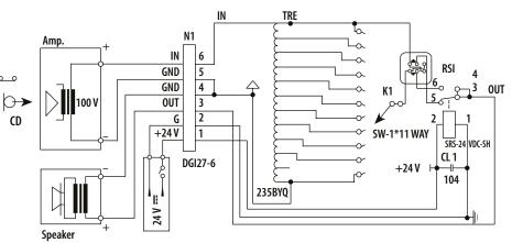
Active mode: Volume control will be fully opened and set to the maximum level until 24V DC is supplied. After DC powering, volume control will come in to operation. Passive mode: Volume control will be active before 24V DC will not supplied. When DC is powered, Volume control will not be active and volume will be set to maximum level.
