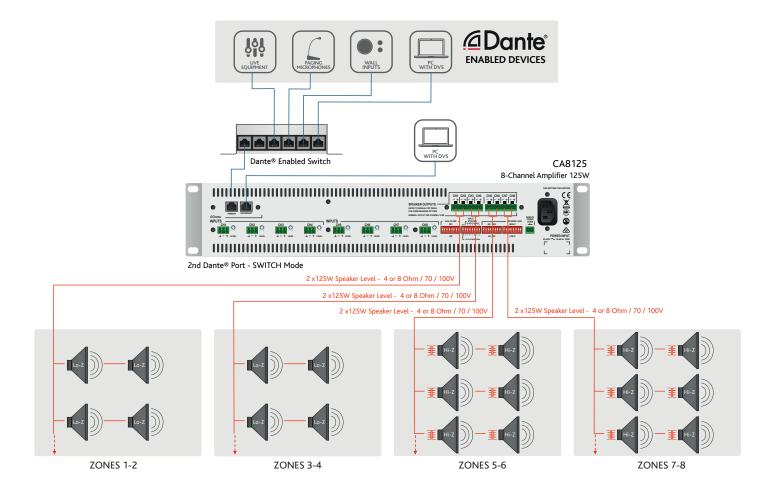
The example above shows an how the eight channels of a CA8125 amplifier may be used to provide stereo audio to different zones of a building. Both 70/100 V-line and low impedance loudspeakers are installed (in different zones), and the system may be extended to additional speakers in each zone as required, provided the total 500 W power capacity of the odd/even channel groups is not exceeded.
