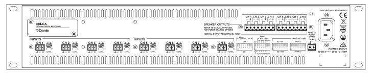
Cloud CA8125 - rear panel view (CA6160/4250/2500 differ only in the number of channels and DIP switch poles)
