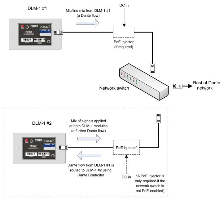
Additional wiring required if a second plate is to be installed in the same zone
