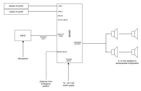
The system shown here uses an MA40F to provide the commentary and music in a mobile tour guiding application, such as on a bus, tram or river boat. The ability of the MA40 range to operate from a low-voltage DC supply makes it particularly useful for this type of application.
