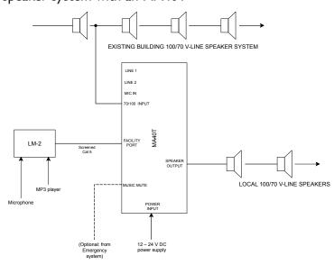
In this example, an MA40T is used to provide local music and microphone amplification in a particular part of a building (possibly a new extension), while at the same time ensuring that the local loudspeakers are integrated with the main building PA/VA system.
