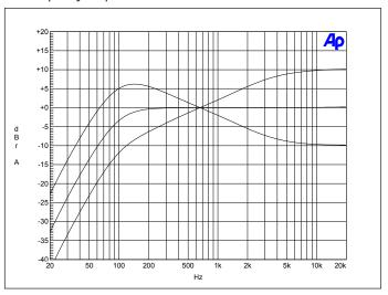
Mic input frequency response, including the rear panel Mic EQ response. Load 8 ohm, middle is flat (MIC LF / HF set to 0) 100 Hz HPF evident
