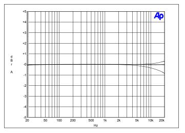
Frequency Response of Line input under 3 different load conditions. 40hm, 80hm & 160hm (from bottom to top) (80hm is flat)
