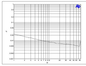
THD+N (%) vs Output Power (W) into a 40hm load. 1kHz sine wave input 20 - 22kHz analyser signal bandwidth
