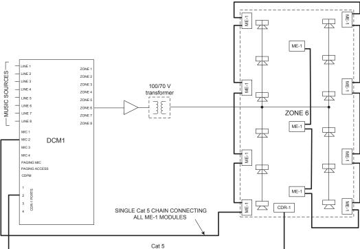
This example shows what might be a large hall or multi-purpose area forming one of the DCMI's zones (Zone 6 in this case). A single CDR-I is fitted at one end to select and control the music routed to the area.
