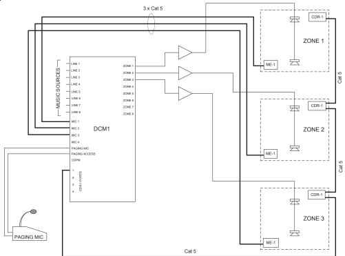
In the system shown, a DCMI is used to route a variety of music sources to three zones. Each zone has a CDR-I remote control plate installed, to allow the users in each area to select the music source and control the volume locally.
