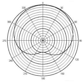
Polar Response Source level: 0.1 Pa Frequency: 1000 Hz
