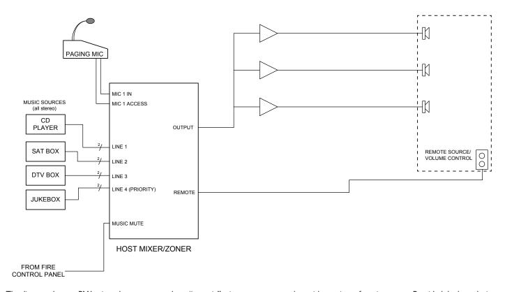
The diagram shows a PMI microphone connected to a "generic" mixer or zoner, together with a variety of music sources. Provided the host device is correctly configured, pressing the PMI's PTT switch will automatically mute the selected music source and allow paging from the microphone.
