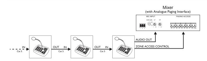
Up to 32 PM Series microphones may be interconnected in a simple "daisy-chain" manner via the Digital Paging Interface, using standard CAT-5 cable and RJ45 connectors. Microphones may be located anywhere in the system, provided that the total cable length does not exceed I km.
