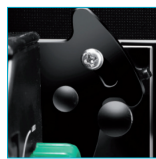
Casing level adjustment
