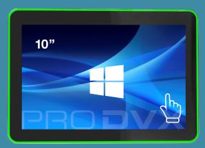
Commercial Grade Intel (X86) Panel PC for Professional usage. Semi High brightness 10.1 inch LCD with Surround LED Bar and Power over Ethernet (PoE). Flat plastic Housing with VESA 75.
