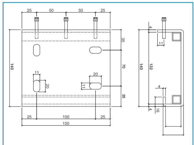
Technical drawing of the ceiling mounting bracket
