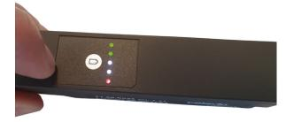
A total of five LEDs are representing the remaining capacity, each represening 20% charge.
