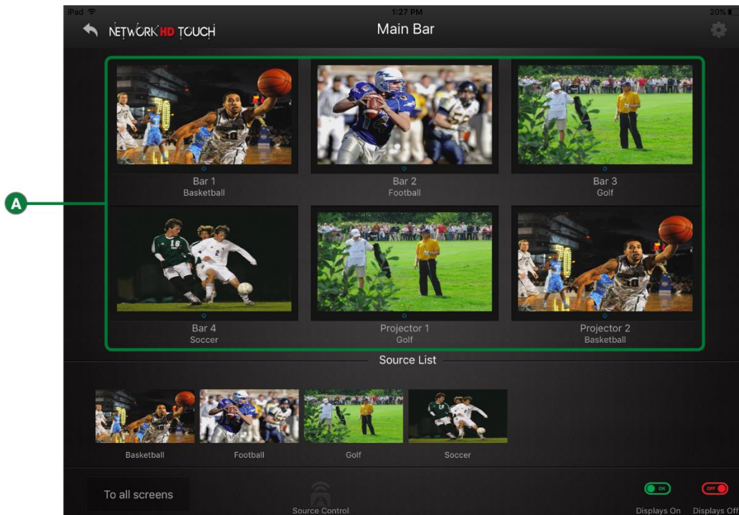
A Matrix Previews Shows a live preview of current matrix assignments. Drag and drop from the Source List to a display to change content.
