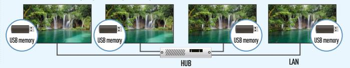
One of up to four display units becomes the parent unit, and the other units display images in sync with the parent unit. This enables the display of images in perfect sync when the panels are arranged next to each other.
